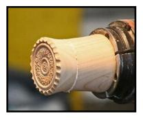
The two beads were formed using a beading tool, the areas inside and between the beads were slightly domed using a beading/parting tool. Nick used a rotating burr to texture between the beads, he used a figure of eight
