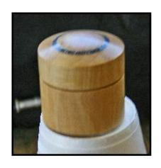
Gary had prepared a piece of Corian by drilling a hole through it, the diameter was about 25mm. He turned a spigot on the box top to fit in the Corian. He used superglue and accelerator to glue the Corian to the box top. With gentle cuts he removed the excess Corian and finished shaping the top.
